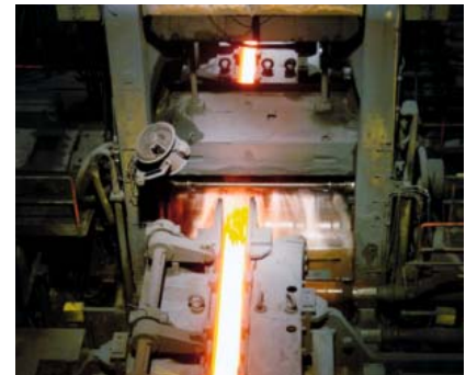
Temperatures must be precisely measured when pressing rails.
